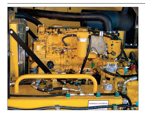
**Turbocharged engine** for top performance and efficiency, even at high altitude with no derating required up to 2134 m (7,000 ft).
