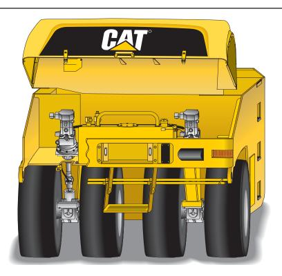
**Hydrostatic transmission** provides smooth direction and speed control, no chains are used.
