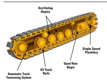
**Quad Rear Bogie.** A special quad bogie is positioned near the rear of the steel track in order to evenly distribute the load.
