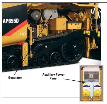
**Industrial, Single-Phase A.C. Generator.** The tractor-mounted generator provides 25 kW of power at 60 Hz for the electric screed heat and the auxiliary power panel. Circuit breaker protection, internal electronic voltage regulation and a dual bearing design provide reliability.
