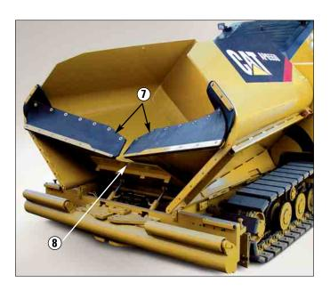
**Precise Mix Delivery.** The material delivery system provides precise mix delivery with minimal operator monitoring. The left and right conveyors in addition to the left and right augers are controlled independently.
