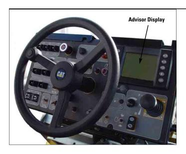
**Advisor Monitoring System (AMS).** The LCD Advisor provides access to a start-up checklist, operator preferences, engine and machine operating parameters and "Paving Calculator".
