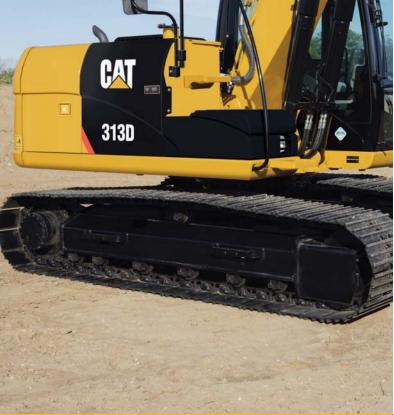
Caterpillar uses advanced engineering and software to analyze all structures, creating a durable, reliable machine for the toughest applications. More than 70 percent of the structural welds are robotic and achieve additional penetration over manual welds. These structural components and undercarriage are the backbone of the machine's durability.
