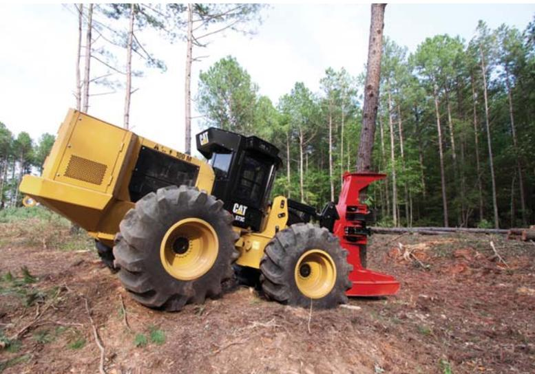
Cat engines, field-proven hydrostatic drive and Cat axles make a solid, responsive power train. A new design to keep the pump drive and gearbox well lubricated provides even more durability.
