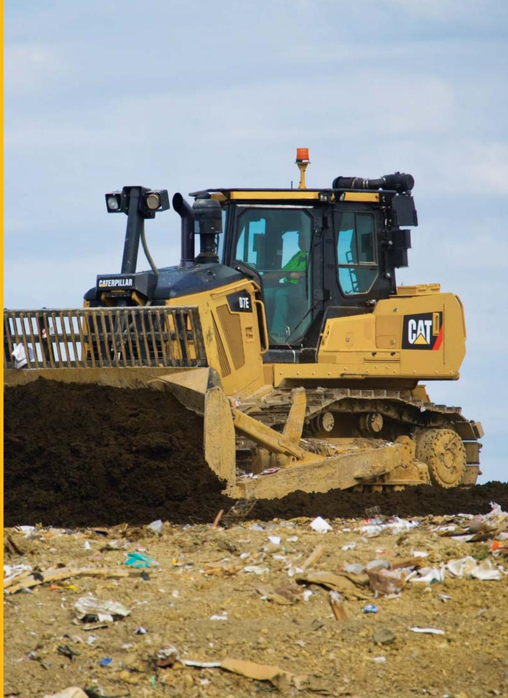
**Like all Cat® waste handlers, the D7E is a heavy-duty machine with specialized guarding designed just for waste handling applications. Its versatility makes it a powerful and highly maneuverable machine for dozing and compacting waste, as well as an ideal fine grading machine to place just the right depth of cover material.**
