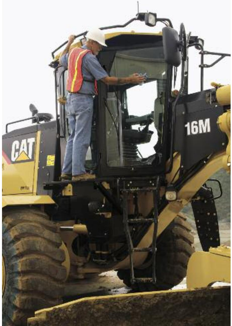
**Additional Safety Features.** The 16M has many additional standard safety features, including laminated glass on the front windows and doors, back-uplights and sounding alarm, black glare-reducing
