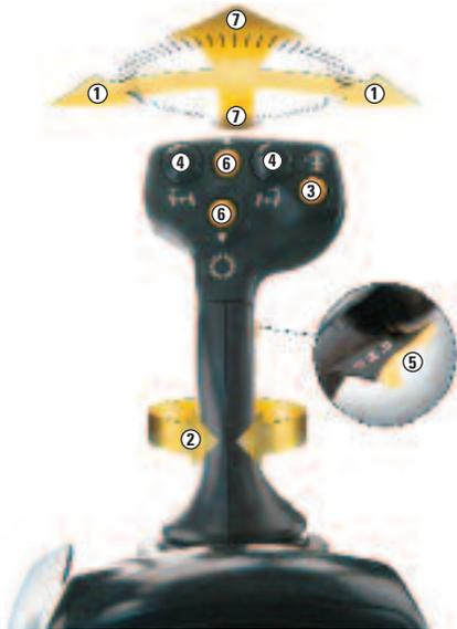
**Left Joystick Functions.** The left joystick primarily controls the machine direction and speed.
