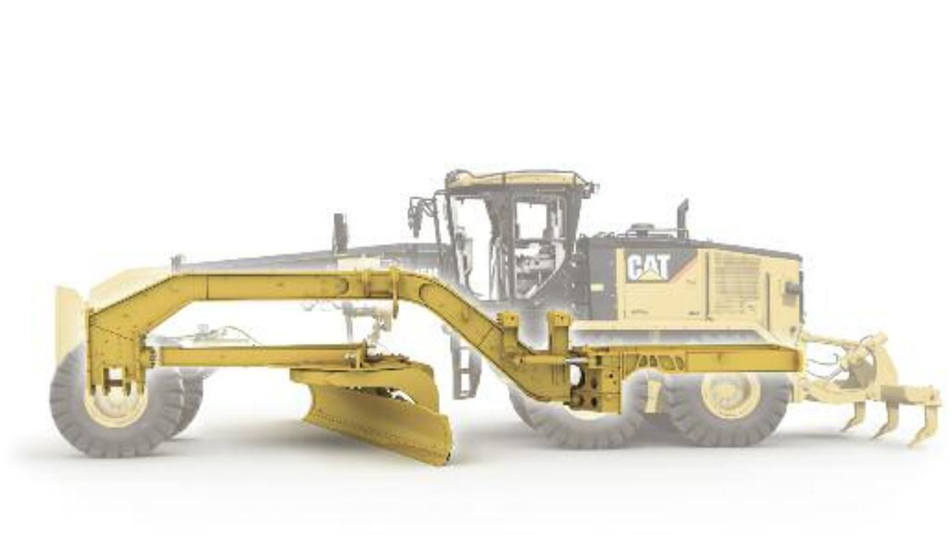
**Front Frame Structure.** Continuous top and bottom plate construction provides consistency and strength. The flanged box section design removes welds from high stress areas, improving reliability and durability, and increasing resale values for the customer.
