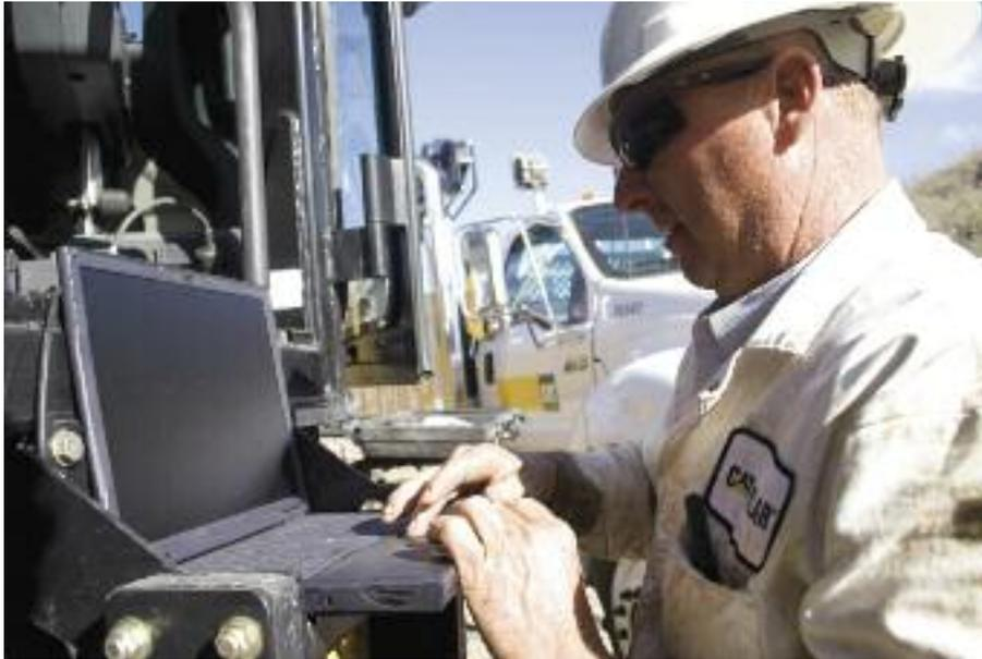
**“Smart Machine”.** The 16M fully integrates all core systems creating a “Smart Machine.” The Cat data link shares key data among systems, optimizing machine performance while preventing potential machine damage.
