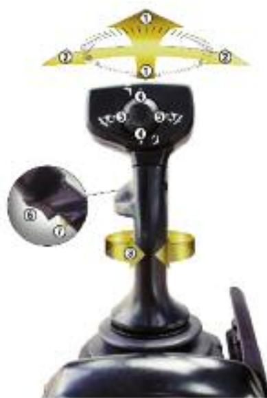
**Right Joystick Functions.** The right joystick primarily controls the Drawbar, Circle and Moldboard functions.
