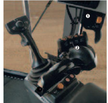
**1 – Ripper Control Pod.** Infinitely variable roller switches control the rear ripper and/or front lift group (when equipped), for easy and comfortable control.
