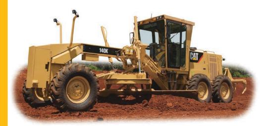
The 140K optimizes your investment by delivering maximum productivity and durability. The Cat C7 engine, direct-drive power shift transmission and load-sensing hydraulics work together to ensure the power and precision to get the job done.
