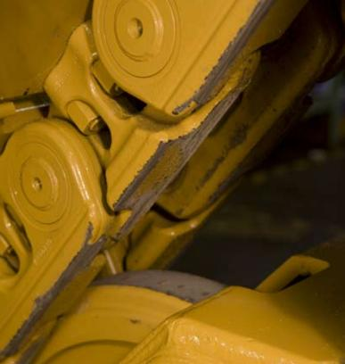
Optional SystemOne<sup>TM</sup> undercarriage offers a variety of features and benefits improving mechanical availability, overall performance of the undercarriage, wear life, and most importantly productivity. This enhanced version of SystemOne<sup>TM</sup> also addresses issues like thrust wear, sprocket segment retention, and dry joints.
