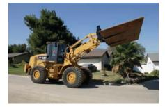
**Load Sensing Hydraulics.** The IT38H features a load sensing hydraulic system that supplies flow and pressure for the implements only upon demand, and only in the amounts necessary to perform the needed work thus providing a more efficient loader.
