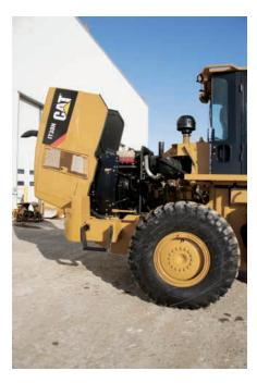
**Engine Compartment Access.** A single mechanical lift cylinder with manual back-up opens the hood. The tilting hood provides excellent access to the engine and cooling compartments and if necessary, the entire hood can be removed with the built-in lift points.
