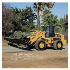
**Forks.** Logging, Millyard and Pallet Forks are available for forestry and material handling applications.
