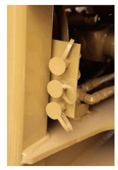
**Remote Pressure Taps.** Pressure taps for key systems are grouped and centrally located throughout the machine and help facilitate quick diagnostics.
