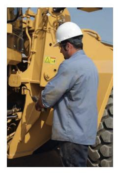
**Ground Level Grease Points.** Grease fittings are grouped throughout the machine thus facilitating easy lubrication of vital components.
