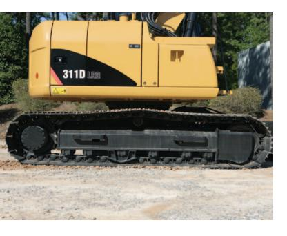
Caterpillar uses advanced engineering and software to analyze all structures, creating a durable, reliable machine for the toughest applications. More than 70 percent of the structural welds are robotic and achieve additional penetration over manual welds. These structural components and undercarriage are the backbone of the machine's durability.
