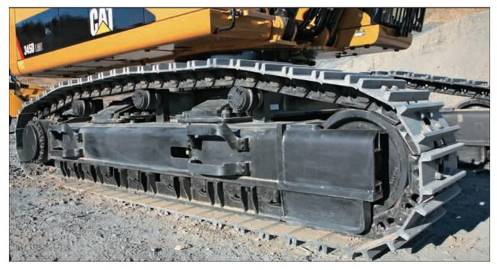
**Undercarriage Options.** The 345D L comes standard with a grease lubricated track called GLT4. The track links are assembled and sealed with grease to decrease internal bushing wear, reduce travel noise, and lower operating costs by extending service life. Track with Positive Pin Retention 2 (PPR2) and Cast Idlers are available as attachments on the 345D L.
