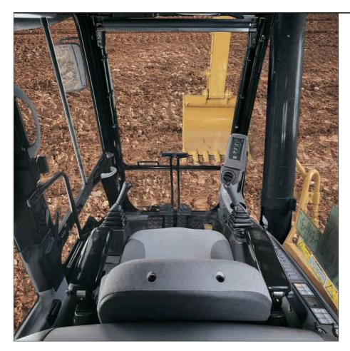
**Cab Design.** The workstation is spacious, quiet and comfortable, assuring high productivity during a long work day. The air conditioner and attachment switches are conveniently located on the right-hand wall, and the key switch and throttle dial are on the right-hand console. The monitor is easy to see with excellent visibility.
