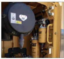
**Extended Service Intervals.** Extended service and maintenance intervals increase machine availability. The maintenance intervals for engine oil, engine oil filter and water separator for fuel line have been extended to 500 hours, hydraulic oil to 2000 hours for normal applications with S•O•S<sup>SM</sup> analysis monitoring.
