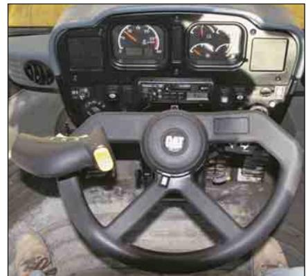
Full machine articulation is accomplished with a  $\pm 70^\circ$  turn of the wheel – versus two to three  $360^\circ$  turns of a conventional steering wheel. The Command Control Steering wheel contains the forward/neutral/reverse switch and the upshift/downshift button – allowing the left hand to remain on the steering wheel at all times. The CCS column inclines  $35^\circ$  and the telescopic change is up to 100 mm.
