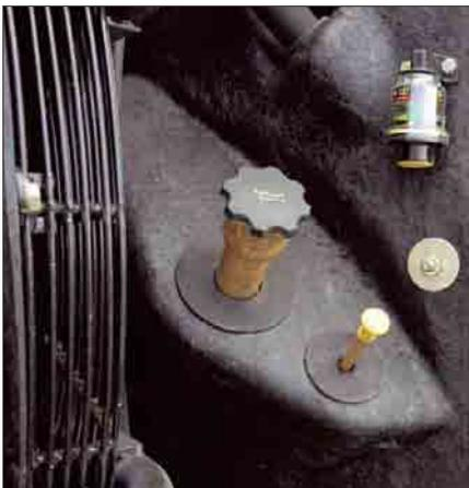
With the hood closed, quick checks of the engine oil level, coolant site gauge and air inlet indicator can be completed through the side service door.
