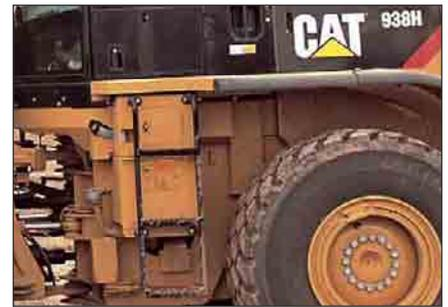
**Entry and Exit.** A ladder with aggressive tread pattern keeps debris build-up to a minimum. The ladder is at a 5° forward incline for easy entry and exit. The main cab door opens a full 180° and latches in place to allow safe navigation to the rear of the machine. The right side door opens 10°, or completely for secondary exit simply by pulling a pin. A full-length ladder on the right side facilitates safe exit if needed.
