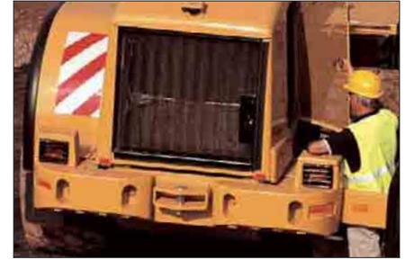
**Counterweight.** The two-piece counterweight is integrated into the 938H design and provides added protection for the lights by incorporating them into the top of the structure.
