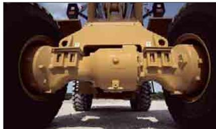
**New! Differential Lock.** Maximize productivity with the new hydraulic locking front differential. This standard feature provides operators with the confidence to maneuver through poor underfoot conditions with 'on the fly' engagement.
