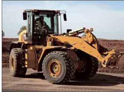
**Steering.** Caterpillar's low effort Load-Sensing steering directs power through the steering system only when needed. The new hand metering unit and priority valve provide operators with full steering and multi-function capability at low engine RPM's. The combined steering column and instrument panel tilt for maximum operator comfort.
