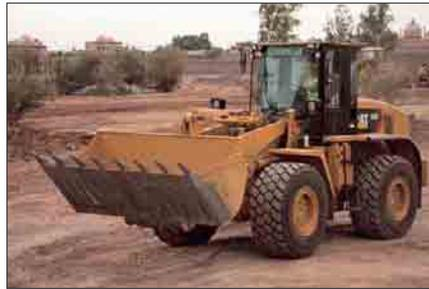
**Constant Net Horsepower.** On many competitive machines, gross horsepower is constant, meaning that net engine power available for actual work will vary based on demands made from parasitic sources, such as air conditioning or cooling fans. The Cat C6.6 engine is electronically configured to provide constant net horsepower at full parasitic load enhancing productivity and improving fuel efficiency.
