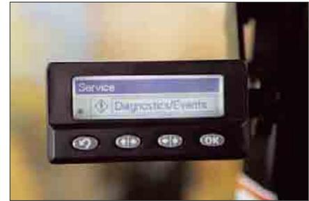
**Cat Messenger.** Messenger offers the comfort of providing real-time, visual feedback on engine and machine operating conditions. It displays information on diagnostic codes, maintenance and system parameters.
