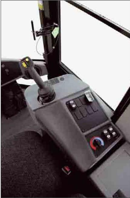
**Implement Control Pod.** The newly restyled implement pod provides superior comfort through the full length adjustable armrest. Standard transmission F-N-R switch allows operators to keep their hand on the implement control levers while making directional shifts. An optional joystick with integrated F-N-R switch is available and replaces the lift and tilt levers.
