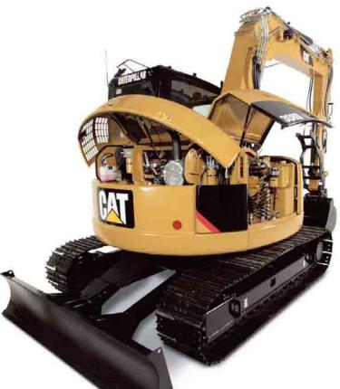
Robust, reliable and easily serviced are the key attributes of Caterpillar Mini Hydraulic Excavators. Full steel body work panels provide durable protection against damage. All daily service points are easily accessed through the rear hood and side cover and a 500 hour engine oil change interval lowers operating costs. The Cat S•O•S. points assist easy oil sampling for preventative maintenance checks.
