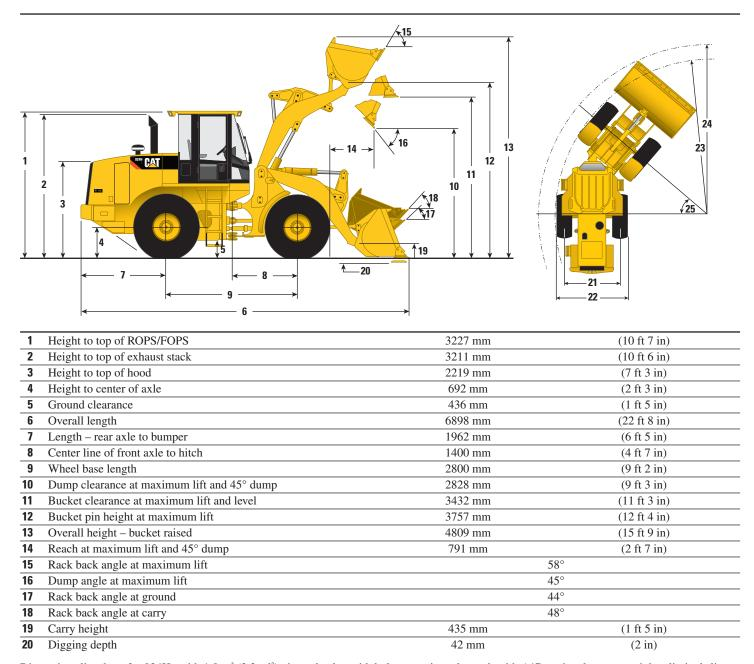
Dimensions listed are for 924Hz with 1.8  $\,\mathrm{m}^3$  (2.3  $\,\mathrm{yd}^3$ ) pin-on bucket with bolt-on cutting edge, cab with A/C, optional counterweights, limited slip axles, heavy duty rear brakes, additional guarding, sound suppression, work tool, 80  $\,\mathrm{kg}$  (176  $\,\mathrm{lb}$ ) operator and Michelin 20.5 R25 L3 XHA tires.
