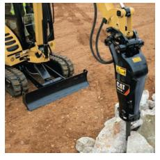
Auxiliary Lines and Connectors. The auxiliary lines and connectors are fitted as standard, meaning the Cat 301.6C and 301.8C come ready to work. Hammer (one-way) auxiliary lines are also fitted as standard.
