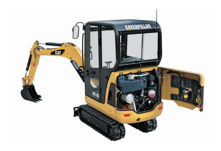
**Front Linkage.** Protected front linkage lines are routed above the boom and stick to help reduce damage and downtime.
