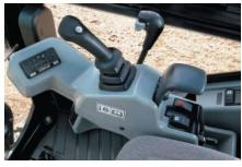
**Low Effort Controls.** Ergonomic, low effort controls offer greater operator comfort for increased productivity. Dozer lever mounted, two-speed travel control provides easy operation and increases foot room.
