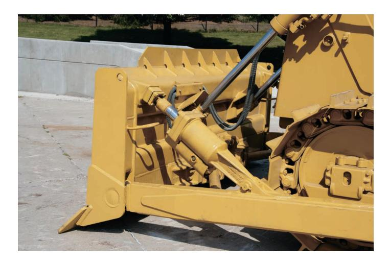
**Bulldozers.** All blades feature a strongbox-section design that resists twisting and cracking. Blades are made of Cat DH-2<sup>TM</sup> steel that has high tensile strength and stands up to the most severe applications. Heavy moldboard construction and hardened bolt-on cutting edges and end bits add strength and durability.
