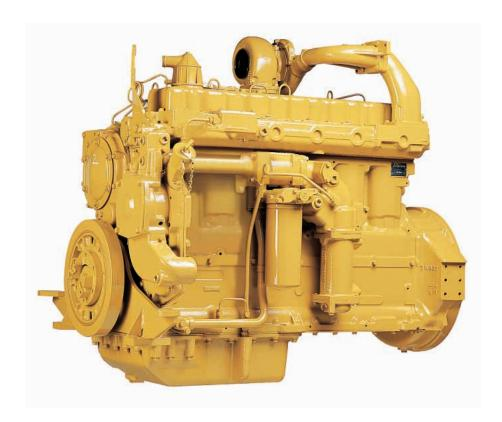
Aluminum Pistons. The 3306 features cam-ground three-ring cast tapered aluminum alloy pistons used to reduce friction, decrease heat build-up and provide excellent oil control. Crankcase journals are hardened and aluminum bearings are steel-backed. The high fatigue aluminum alloy-bearings surface not only has the capability to withstand heavy shock loads during crankshaft rotation, it will also adapt to normal wear of the crankshaft journals.
