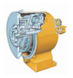
**Torque Divider.** The torque divider arrangement is a Caterpillar exclusive that provides high torque multiplication when under load with direct drive efficiency when completing lower engine load functions such as backfilling trenches or spreading material.
