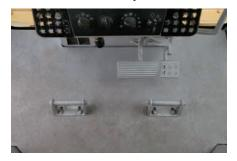
**Brake Pedal.** A single brake pedal actuates both tracks to make operation easier.
