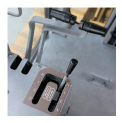
**Directional Controls.** Steering and transmission controls are located conveniently to the operator's left for comfortable operation.
