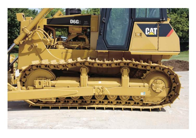
**Roller Frames.** The track roller frame is a reinforced box section construction with seven lifetime lubricated track rollers per side and outside mounted carrier rollers, two per side.
