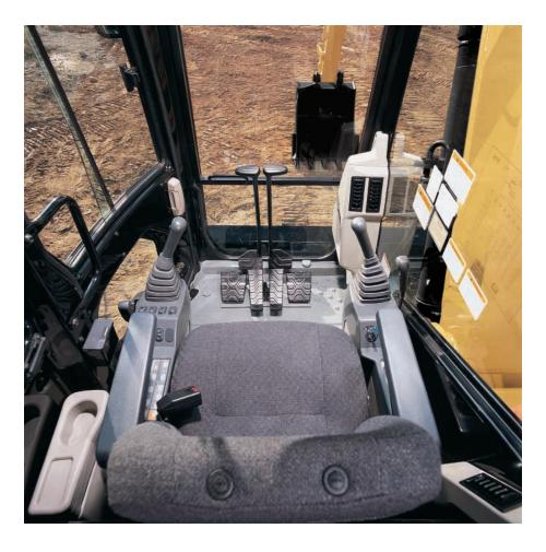
**Cab Design.** An enlarged cab with curved styling gives the operator a comfortable, spacious working environment and improved visibility.
