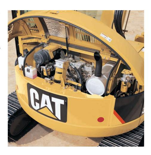
**Cooling System.** A large-diameter fan and full-length, water-cooled cylinders, combined with excellent thermal efficiency, help prevent overheating. The result is longer engine life and the ability to operate at high temperatures and under heavy loads. A mixed flow fan design provides high cooling efficiency. The core radiator is equipped with waved fins to prevent clogging.
