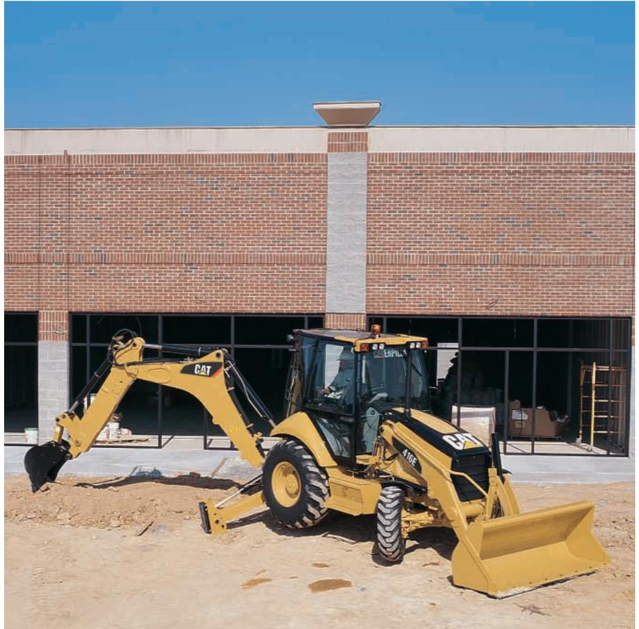
**Flip Over Stabilizer Pads.** Flip over stabilizer pads provide the ability to work in both dirt and street applications. New pads are stronger, feature a positive anti-flip mechanism and provide increased rubber wear life.
