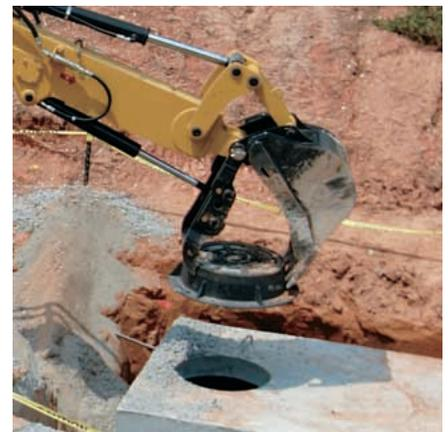
**Thumb.** Available for both the standard and the extendible stick, thumbs increase the versatility of the backhoe with the ability to grip, grab and sort virtually any material.
