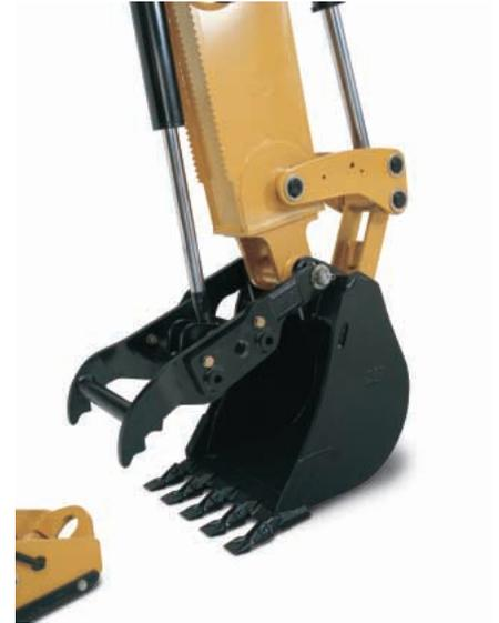
**Thumb Mounting.** Thumb mounting provisions are standard on every Cat Backhoe Loader for added machine versatility. Hydraulic thumbs are available factory-installed.
