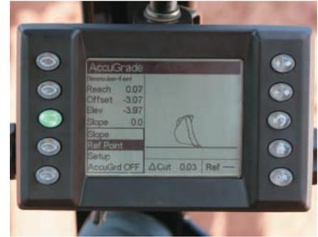
**In-Cab Display.** The AccuGrade monitor allows the operator to enter slope and dig depth parameters. The in-cab display with easy to read grade indicator and elevation display delivers all system information to the cab for easy viewing by the operator.
