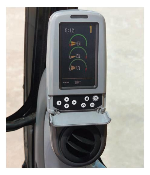
**Monitor Display Screen.** The monitor is a full color 400 x 234 pixels Liquid Crystal Display (LCD) graphic display.
