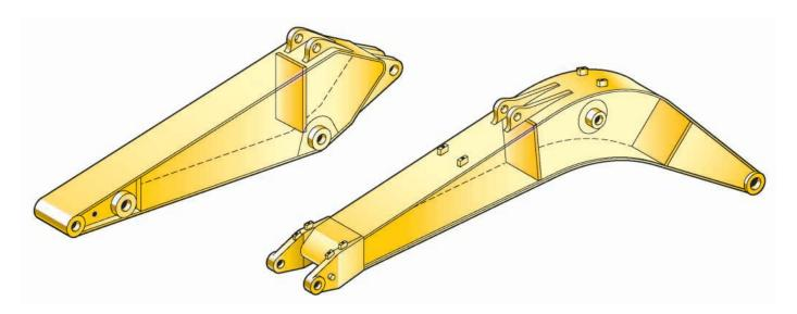
Front Linkage Attachments. Select the right combination of front linkage with your Cat dealer to ensure high productivity from the very start of your job. Three types of booms and six sticks are available, offering a range of configurations suitable for a wide variety of applications. The 385C L offers a large combination of reach and digging forces for optimum versatility.
