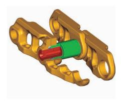
**Track.** The 385C L comes standard with the new grease lubricated track called GLT4. The track links are assembled and sealed with grease to decrease internal bushing wear, reduce travel noise and extend service life lowering operating costs.
