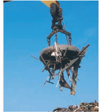
Walker Scrapmaster Series Scrap Handling Magnets. The magnets feature cast steel case and alloy steel suspension chain.
