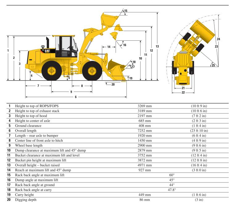
Dimensions listed are for 928Hz with  $2.0~\text{m}^3$  ( $2.6~\text{yd}^3$ ) pin-on bucket with bolt-on cutting edge, cab with A/C, optional counterweights, limited slip axles, heavy duty rear brakes, additional guarding, sound sppression, work tool, 80~kg (176 lb) operator and Michelin 20.5R25~L3 XHA tires.
