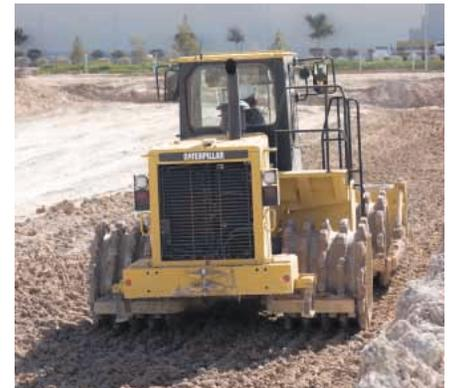
**Cleaner Bars.** Help keep the drums free of carry-over dirt regardless of rolling direction. A pass-through bolt design allows for easier serviceability.
