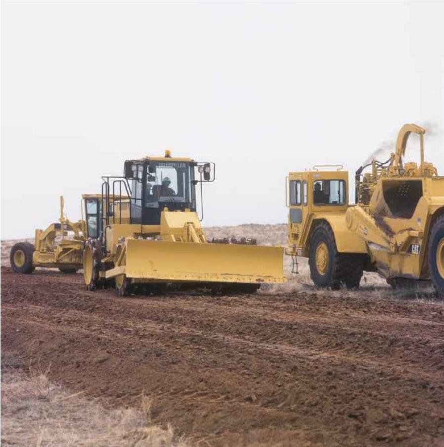
**Blade Package.** Consists of the blade, push-arms, trunnion mounting, dozer-length skid plate with replaceable wear plates, reversible cutting edges, self-sharpening end bits, hydraulic lines guard and hydraulic lift cylinders.
