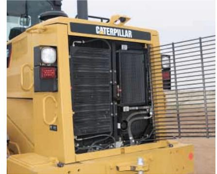
**Hinged Hydraulic Oil Cooler.** Can be swung open without special tools.
