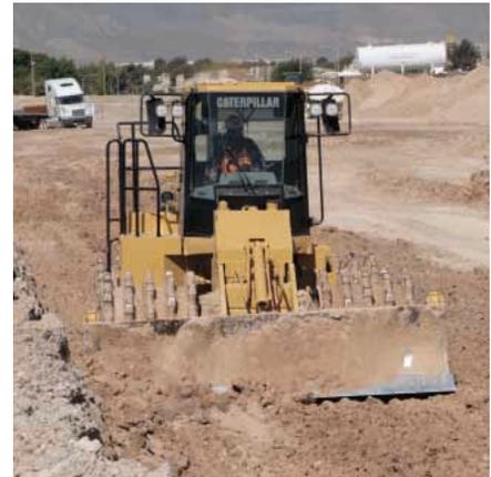
**Applications.** The 815F Series 2 excels at compacting, spreading fill, backfilling and boosting scrapers. With the ability to work at higher speeds over other types of soil compactors, the 815F Series 2 can keep up with a fast-moving scraper fleet or an articulated truck hauling operation. When speed and dozing capability are required job duties for a soil compactor, the 815F Series 2 has no equal.
