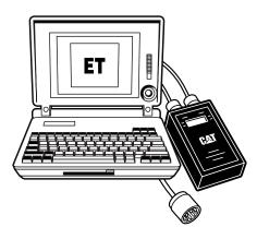
**Cat Electronic Technician (ET).** Is a software program which allows the service technician to find and identify a problem on a machine and to analyze how to fix it quickly. Cat ET provides the capability to access the electronic control modules from a personal computer.
