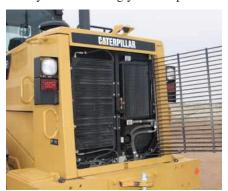
Hinged Hydraulic Oil Cooler and Air Conditioning Condenser. Swing open without special tools and allows the cooling system to be cleaned quickly and easily.
