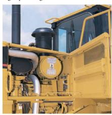
**Right Side Service Access.** Features that are easily reached under the hood include fuel filter and water separator, fuel primer and engine oil dipstick.
