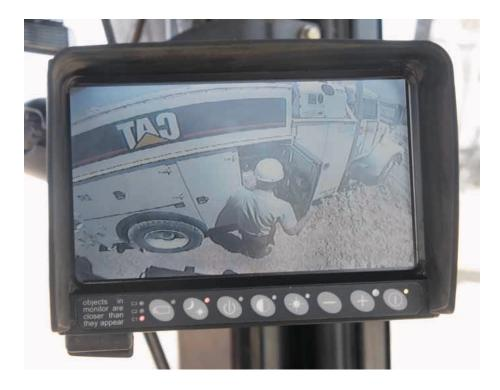
**Rear Vision Camera.** Uses a camera mounted on the radiator guard and a monitor in the cab to allow the operator to see the area directly behind the machine.
