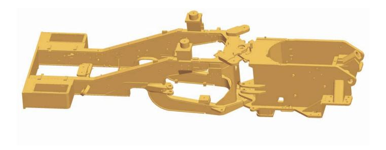
Structure Construction. Combines the use of robotic welding on up to 90 percent of the 814F Series 2 with castings in several areas to increase strength by helping spread the loads and reduce the number of parts. This provides highly consistent welds with deep plate penetration and excellent plate fusion. The benefits are increased durability and fatigue strength. The computer controlled machining ensures the alignment of pin bore, axle pad, cab mount and transmission/engine components.
