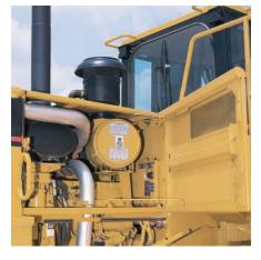
**Right Side Service Access.** Features that are easily reached under the hood include fuel filter and water separator, fuel primer and engine oil dipstick.
