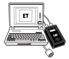
**Cat Electronic Technician (ET).** Is a software program which allows the service technician to find and identify a problem on a machine and to analyze how to fix it quickly. Cat ET provides the capability to access the electronic control modules from a personal computer.
