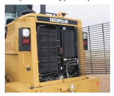
Hinged Hydraulic Oil Cooler and Air Conditioning Condenser. Swing open without special tools and allows the cooling system to be cleaned quickly and easily.
