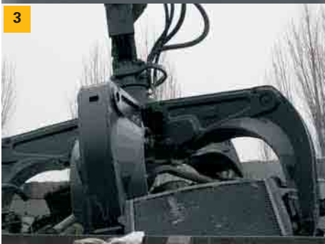
1 Bulk handling for inland waterways application 2 Machine monitoring control 3 Scrap handling application, orange peel grapple
