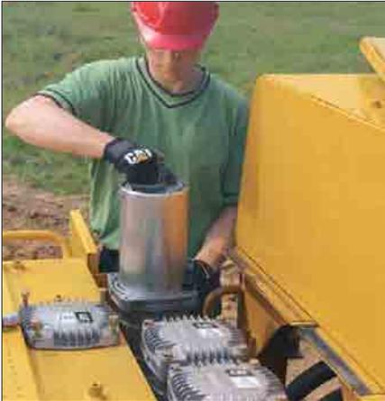
**Service Intervals.** Service intervals are extended to reduce maintenance costs. Engine oil, oil filter and fuel filters at 500 hours.
