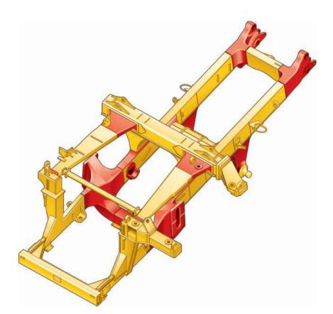
**Box-Section Design.** The 777F frame uses a steel box-section design, incorporating two forgings and 19 castings in high-stress areas with deep penetrating and continuous wrap-around welds to resist damage from twisting loads without adding extra weight.
