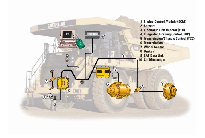
**Cat Data Link.** Electronically integrates machine computer systems to optimize overall power train performance, increase reliability and component life, and reduce operating costs. All control modules communicate via the Cat Data Link and work together as an integrated system to maximize production efficiency and extend component life.
