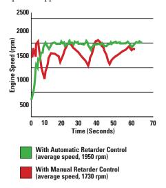
• **Faster Speeds.** ARC allows the operator to maintain optimum engine speeds for up to 15 percent faster downhill hauls and greater productivity.
