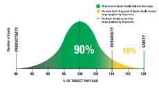
**Target Payload Strategy**. Your Caterpillar Dealer can help you manage to target payload to maximize equipment use, ensure safe operation, increase productivity and lower cost-per-ton.
