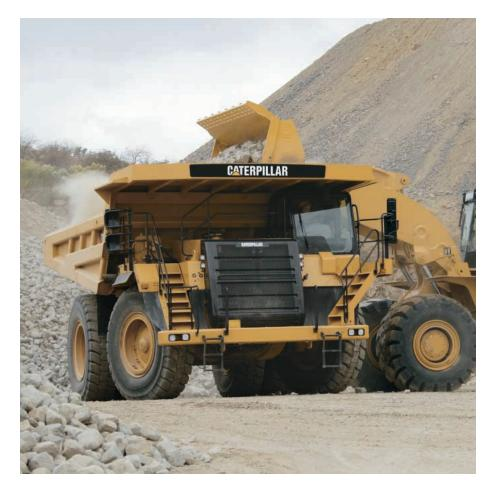
• Overloading causes excessive wear on vehicle components, such as brakes, tires and drive train, reducing component life and increasing maintenance costs and repairs. **Matched Systems.** Designed to work as an optimum pass/match system, the 777F is best sized to match the 990H Wheel Loader, with a 6 pass/match, and the 992G Wheel Loader, with 4 pass/match.
