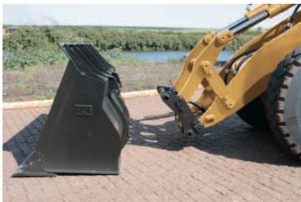
**Quick Couplers.** Quick couplers provide unmatched versatility for wheel loaders. The hydraulic model allows an operator to change attachments in seconds without leaving the cab. On the manual model, the operator must lock the pins.
