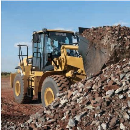
**LOAD SENSING HYDRAULICS.** The IT62H features a load sensing hydraulic system that automatically adjusts to operating conditions to provide only the hydraulic flow requested by the operator for improved fuel efficiency.
