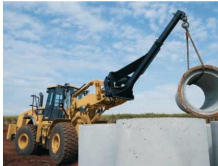
**Material Handling Arms.** Material Handling Arms move pipe, concrete blocks, highway dividers and other construction materials quickly and precisely.
