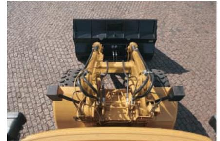
**8-Bar Linkage.** This linkage provides parallel lift to keep the load level throughout the lift cycle – particularly important when using forks. Parallel lift allows the operator to concentrate on placing the load, instead of retaining it. Visibility to the work tool is excellent.
