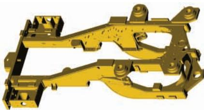
**Engine End Frame (EEF).** A full box-section engine end frame with hitch plates at the front end provides a strong, rigid structure that resists twisting and impact loads. The result is an extremely solid mounting platform for the engine, transmission, axle, ROPS and other accessories.
