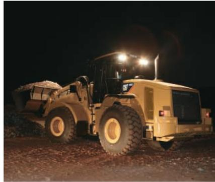
**Lighting Packages.** Optional lighting packages are available for roading or low-light applications. The optional High Intensity Discharge (HID) lights provide exceptional lighting for night work. A rotating beacon is available as a safety feature.
