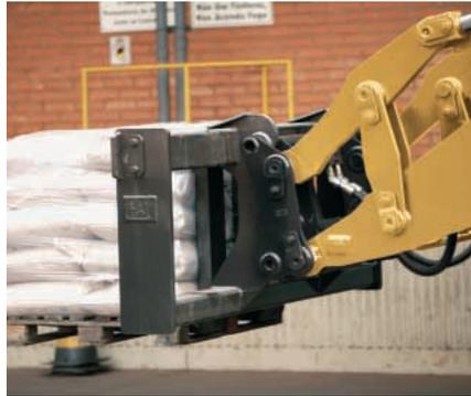
**Pallet Forks.** When used with a quick coupler, pallet forks increase the versatility of the machine; ideal for handling a variety of materials.
