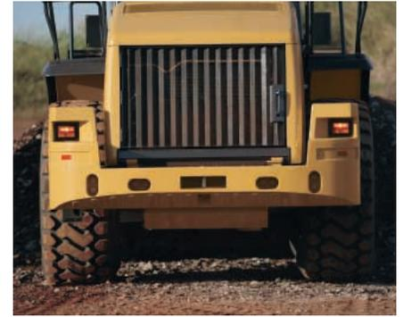
**Counterweight.** The one-piece counterweight is integrated into the IT62H design and styling. This 4389 lb (1991 kg) counterweight incorporates the rear lights into the top of the structure.
