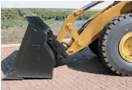
**Material Handling Buckets.** The material handling bucket is a flat-floor bucket used for handling stockpiled materials such as aggregates or other easy-to-load materials requiring moderate breakout force.
