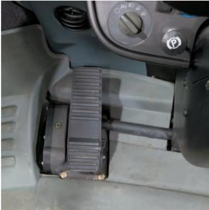
**Integrated Braking System.** The Cat exclusive Integrated Braking System reduces axle oil temperatures and improves transmission neutralizer smoothness. IBS has a direct impact on durability of the axles and brakes especially in applications involving long distances and/or heavy braking.
