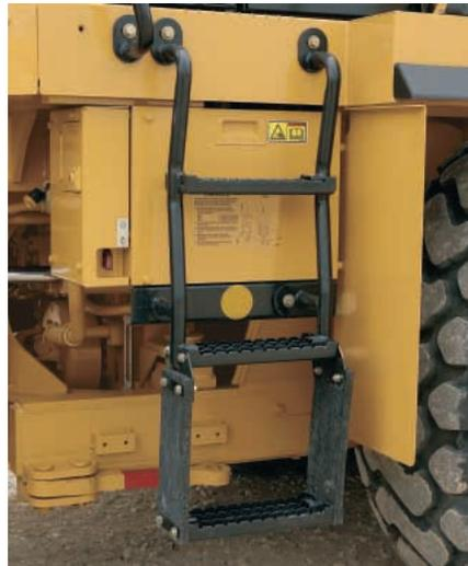
**ENTRY AND EXIT.** An open ladder design keeps debris build-up on the steps to a minimum. The ladder is at a 5° forward incline for easy entry and exit.
