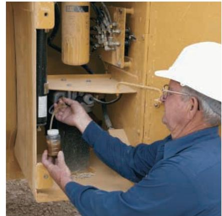
**S•O•S SERVICES.** Sampling valves on the IT62H allow quick access to engine, transmission and hydraulic oils for S•O•S analysis. Oil change intervals and other services can be optimized according to your work schedule, reducing downtime and managing expenses.
