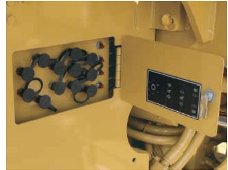
**REMOTE PRESSURE TAPS.** Pressure taps for the steering and hydraulic systems, transmission (optional) and brakes are grouped behind an access panel just below the right-side service platform.
