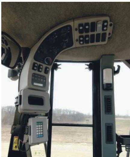
**CONTROLS.** The main control panel on the IT62H is located high on the right ROPS post – keeping everything within reach of the operator while maintaining visibility to the ground. Keeping all switches and controls conveniently placed allows better efficiency and improved productivity all while minimizing operator fatigue. The front dash panel is conveniently laid out for easy monitoring of gauges and operation of controls.
