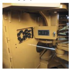
**REMOTE PRESSURE TAPS.** Pressure taps for the steering and hydraulic systems, transmission (optional) and brakes are grouped behind an access panel just below the right-side service platform.
