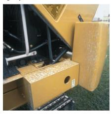
A single mechanical lift cylinder with manual back-up opens the hood. The tilting hood provides excellent access to the engine compartment, and if necessary, the entire hood can be removed with the built-in lift points.
