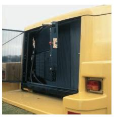
**COOLING SYSTEM.** Cooling system access for clean-out and maintenance is outstanding. The perforated and corrugated grill minimizes debris build-up and swings out for easy cleaning and access to the cooling cores.
