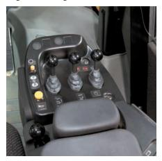
**Seat.** The Cat C-500 Series Comfort air suspension seat, standard in the 966H, is built strong and durable and is 6-way adjustable to accommodate all-sized operators. The cast one-piece back and seat pan prevent protrusions under the cushions. The seat features an automotive-style lumbar support for maximum comfort. The right hand armrest with integrated implement controls adjusts for comfortable, convenient operation. A heated seat option is available for additional comfort.
