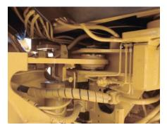
**Spread Hitch.** The distance between the upper and lower hitch plates is an important contributor to machine performance and component life. The Caterpillar spread hitch design provides excellent load distribution and bearing life. Both the upper and lower hitch pins pivot on double tapered roller bearings – improving durability by distributing both vertical and horizontal loads over a larger surface area. The wide opening also provides excellent service access.
