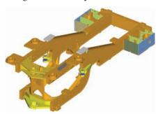
**Engine End Frame (EEF).** A full box-section engine end frame with hitch plates at the front end provides a strong, rigid structure that resists twisting and impact loads. The result is an extremely solid mounting platform for the engine, transmission, axle, ROPS and other accessories.
