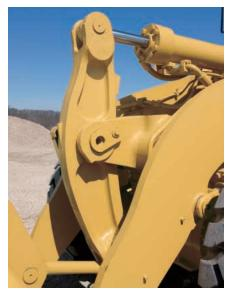
**Linkage.** The 966H linkage is a single-tilt Z-bar design. Z-bar linkage generates excellent breakout force and good rack back angle for better bucket loading and load retention.
