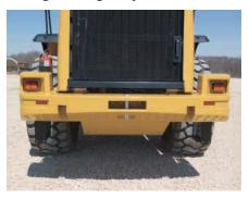
**Counterweight.** The one-piece counterweight is integrated into the 966H design and styling. This 2,517 lb (1142 kg) counterweight incorporates the rear lights into the top of the structure.
