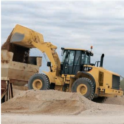
**LOAD SENSING HYDRAULICS.** The 962H features a load sensing hydraulic system that automatically adjusts to operating conditions to provide only the hydraulic flow required by the implement for improved fuel efficiency.
