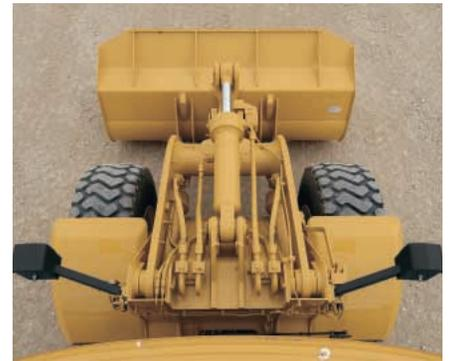
**Linkage.** The 962H linkage is a single-tilt Z-bar design. Z-bar linkage generates excellent breakout force and good rack back angle for better bucket loading and load retention.
