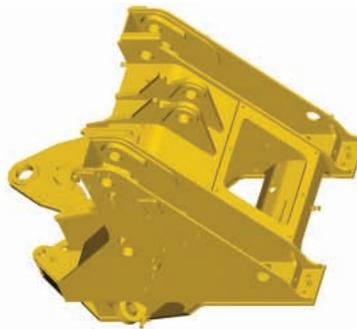
**Non-Engine End Frame (NEEF).** The non-engine end frame provides a solid mounting base for the front axle, lift arms, lift cylinders and tilt cylinders. The fabricated, four-plate loader tower absorbs the forces associated with loading, twisting and penetration.
