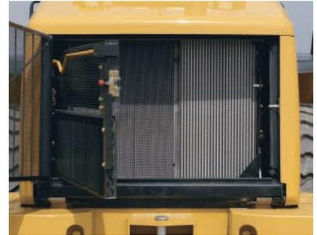
**COOLING SYSTEM.** Cooling system access for clean-out and maintenance is outstanding. The perforated and corrugated grill minimizes debris build-up and swings out for easy cleaning and access to the cooling cores.
