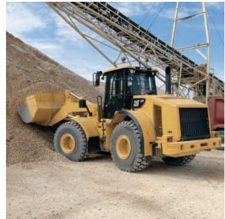
**PLANETARY POWERSHIFT TRANSMISSION.** The electronic planetary powershift transmission with automatic shift capability is designed and built by Caterpillar. The very responsive, full-power speed and directional changes provide excellent cycle times and productivity.
