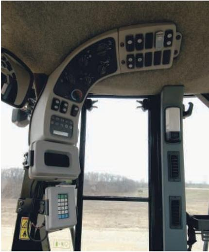
**CONTROLS.** The main control panel on the 962H is located high on the right ROPS post - keeping everything within reach of the operator while maintaining visibility to the ground. Keeping all switches and controls conveniently placed allows better efficiency and improved productivity all while minimizing operator fatigue.
