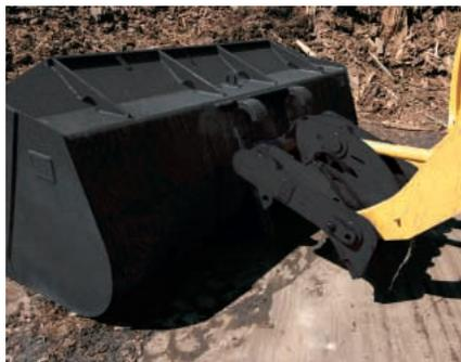
**General Purpose Buckets.** General purpose buckets provide good all-around performance for stockpiling, rehandling, excavating and bank loading. A heavy duty general purpose bucket can be used for more aggressive applications.
