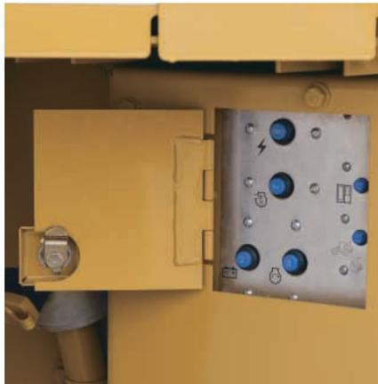
**ELECTRIC SERVICE CENTER.** Batteries, relay panel and an optional tool box are conveniently located below the left-side access platform. The engine shutdown switch is housed with the relay panel. A compartment integrated into the access platform contains the hood tilt actuation switch, master switch and jump-start receptacle.
