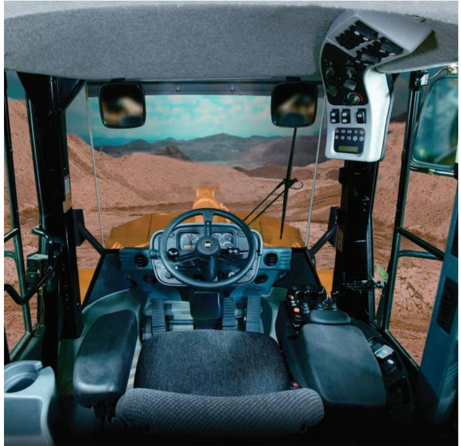
**Command Control Steering.** Command Control Steering is a load-sensing system that links the steering wheel and frame angle positions to provide the proper amount of steering control. The speed the machine turns is proportional to the steering wheel position. Less than 6 lb (26 N) steering effort is required by the operator, regardless of conditions. Full machine articulation is accomplished with a  $\pm 70^\circ$  turn of the
