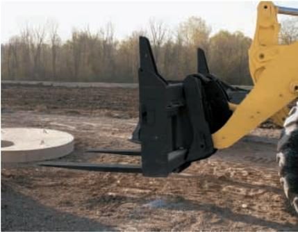
**Forks.** From pallet forks up through specialized logging arrangements, loader forks are available for a wide range of jobs.
