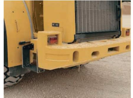
**Counterweight.** The one-piece counterweight is integrated into the 962H design and styling. This 3084 lb (1399 kg) counterweight incorporates the rear lights into the top of the structure.
