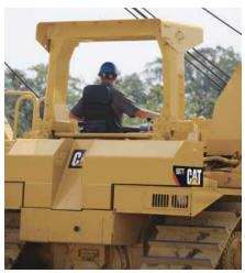
**Optional Roll Over Protective Structure.** Provides increased operator protection.
