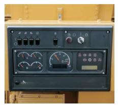
**Monitoring System.** Provides the operator instant feedback on the condition of operating systems and records such performance data as high/low gauge readings to help diagnose problems and manage undercarriage. Has gauges that monitor the temperature of the engine coolant, hydraulic oil and power train oil, plus the fuel level. Also has a digital and gauge type tachometer.
