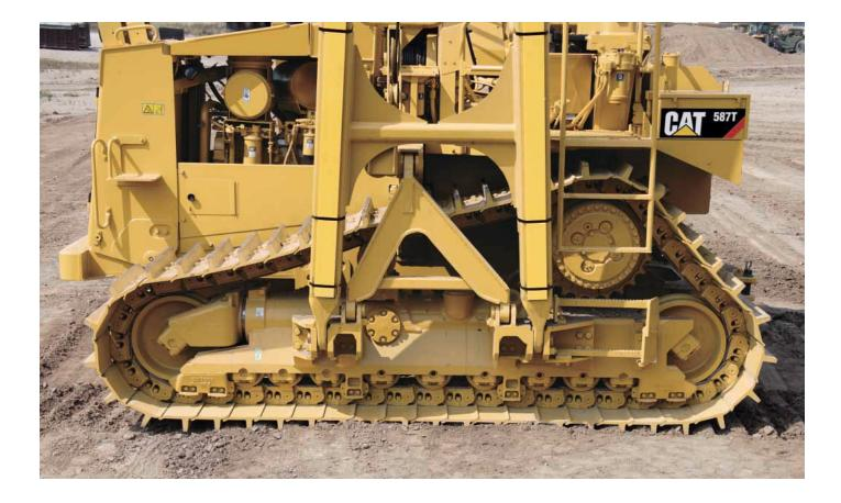
**Final Drives.** Final drives and associated power train components are raised above the work area, isolating them from ground induced impact loads, as well as pipelayer loads, extending power train component life.
