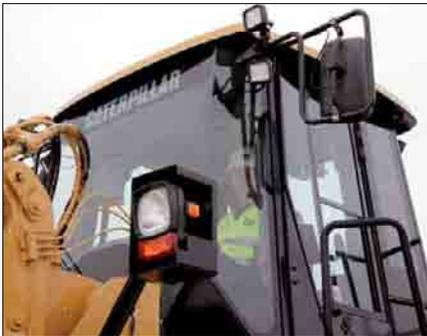
**Visibility.** The IT62H provides excellent visibility to both the front and rear of the machine. The cab has been raised by 50 mm for unmatched visibility. Excellent Visibility throughout the working range with optimized hydraulic hoses routing. Distortion-free flat glass stretches to the floor of the cab for excellent visibility to the bucket. Wet-arm wipers on both front and back keep the windows clean in any
