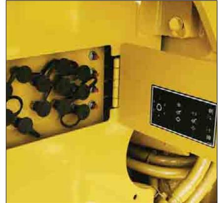
**Remote Pressure Taps.** Pressure taps for the steering and hydraulic systems, transmission and brakes are grouped behind an access panel just below the right-side service platform.
