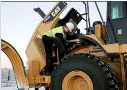
A single mechanical lift cylinder with manual back-up opens the hood. The tilting hood provides excellent access to the engine compartment, and if necessary, the entire hood can be removed with the built-in lift points. With the hood closed, quick checks of engine oil level and the coolant sight gauge can be completed through the side service doors.
