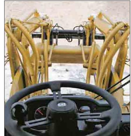
**Front Frame.** The front frame provides a solid mounting base for the front axle, lift arms, lift cylinders and tilt cylinder. The fabricated, four-plate loader tower absorbs the forces associated with loading, twisting and penetration.
