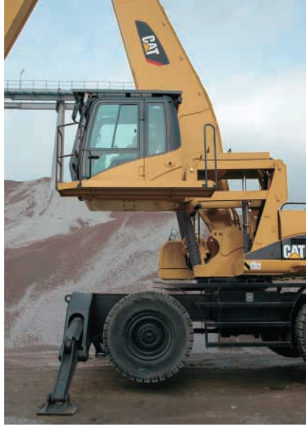
The medium position places the cab forward by 500 mm (20") more than the bottom position for increased visibility.
