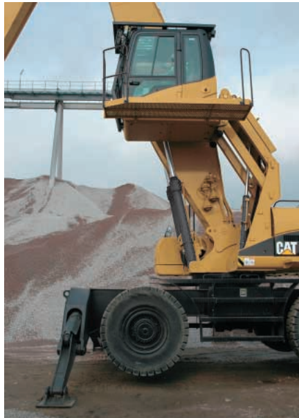
The top position raises the cab by 2.6 m (8'6"). This provides optimum viewing to all sides.
