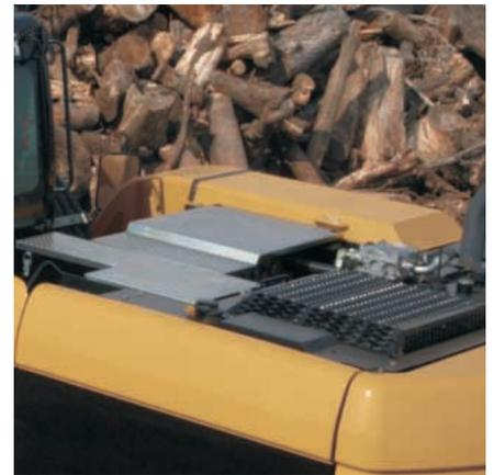
**Anti-Skid Plate.** They cover the top of the steps and upper structure to help prevent slipping during maintenance. The Anti-Skid plate reduces the accumulation of mud on the upper structure, improving the cleanliness and safety.
