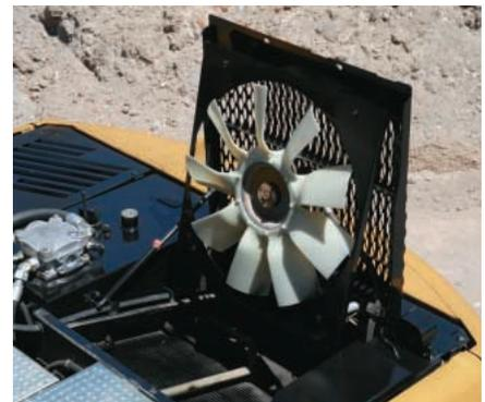
**Easy to Clean Coolers.** Flat fins on all coolers reduce clogging, making it easier to remove debris. The main cooling fan and air conditioner condenser are both hinged for easier cleaning.
