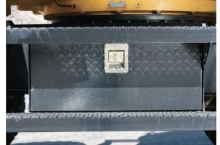
**Storage Box.** There are two toolboxes integrated in the steps of the undercarriage. Additionally, there is a waterproof storage box integrated into the upper structure steps.
