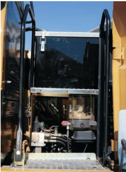
**New Auto-Lube System.** The new automatic lubrication system provides the optimal amount of grease to all the main lubrication points, including the bucket linkage. The lubrication interval can be adjusted through the monitor, and status messages for the auto-lube system are displayed.
