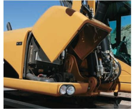
**Front Compartment.** The front compartment hood can be opened vertically, providing outstanding ground level access to the batteries, air-to-air after cooler, air conditioner condenser and the air cleaner filter.
