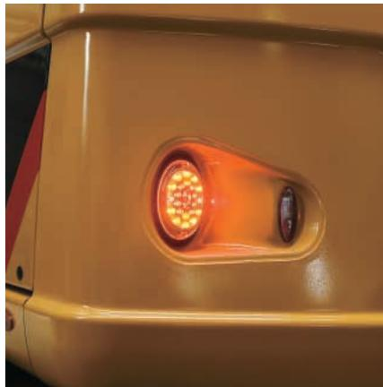
**New LED Rear Lights.** Optional Light Emitting Diode (LED) Rear Lights replace the standard lights, for increased visibility on the job site, higher durability and longer life.
