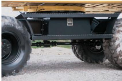
**Drive Line Concept.** The rear mounted transmission and robust drive line design, delivers excellent ground clearance for all off-road applications.
