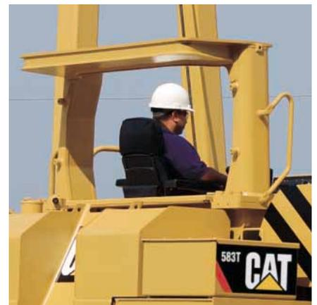
**Optional Rollover Protective Structure.** Provides increased operator protection.
