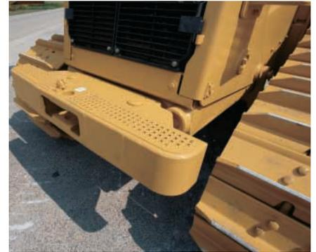
**Front Bumper.** A front bumper is pinned on the frame rails and provides both protection and a towing device. Pipelayer frame mounts are also an integral part of the frame.
