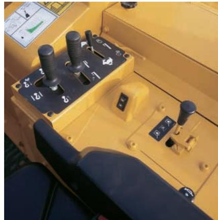
**Ergonomic Work Tool Controls.** Pipelayer controls are low effort and allow simultaneous, precise positioning of the load line and boom with one hand.
