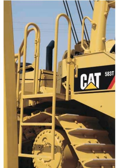
**Access Ladder.** Direct access to the operator's station utilizing ladder on left side of the machine.
