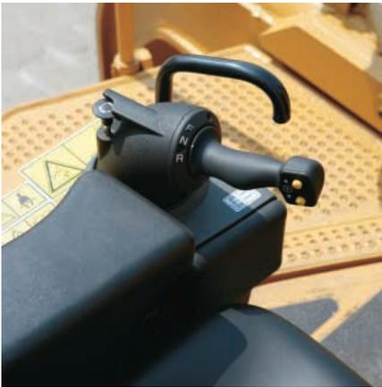
**Steering Control.** Dual-twist tiller control with standard differential steering controls direction and degree of turns, forward-reverse shifting, and gear selection in a single control handle. One hand steering enhances operator comfort.
