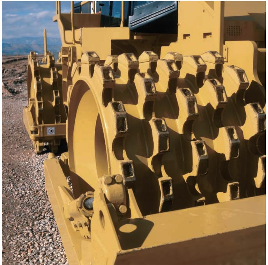
**Standard Tips.** Standard tips are used in typical soil compaction applications where compaction specification requirements are 95-100 percent Standard Proctor. Tip height is 188.3 mm (7.4 in) and tip width is 224 mm (8.8 in).
