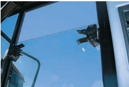
**Optional Sliding Cab Window.** Located in the right and left doors are optional sliding windows to provide access to outside air without opening the door.
