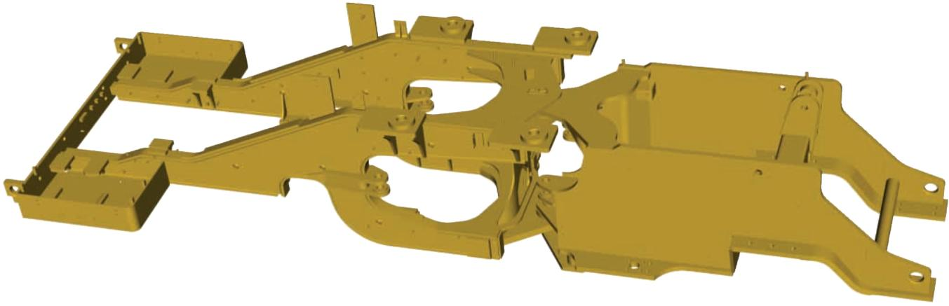
**Structure Construction.** Combines the use of robotic welding on up to 90 percent of the 825H, while castings are used in several areas to increase strength by helping to spread the loads and reduce the number of parts. This provides highly consistent welds with deep plate penetration and excellent plate fusion. The benefits are increased durability and fatigue strength. The computer controlled machining ensures the alignment of pin bore, axle pad, cab mount and transmission/engine components.
