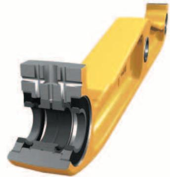
**Equalizer Bar.** The pinned equalizer bar gives the roller frames the ability to oscillate up or down to better match ground contours while providing maximum traction and operator comfort. Equalizer bar with optional oil filled end pin joints and limited slip seals offer longer life in severe applications and reduced repair costs.
