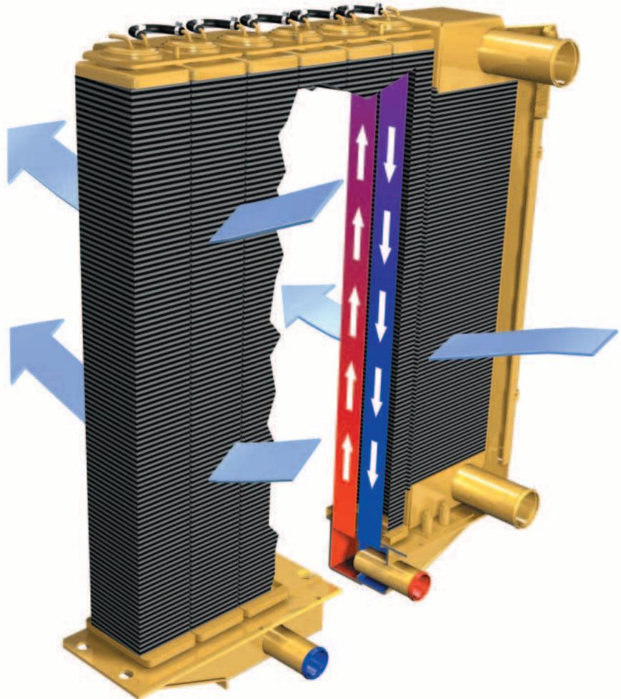
**Protection From Leaks.** To reduce the potential for coolant leaks, brass tubes are welded to a large, thick header, improving strength of the tube-to-header joint. In conditions where abrasive materials can be airborne, use the attachment sand blast grid to prevent core damage.
