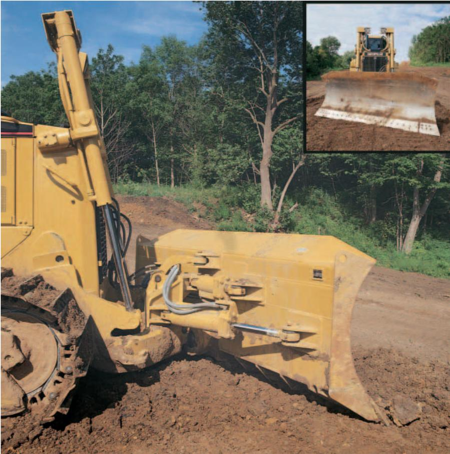
**Caterpillar Blades.** With superior moldboard and cell structure design, Cat bulldozer blades load easily and are durable. Cat high-tensile strength blades resist torsional bending and deflection in tough applications.
