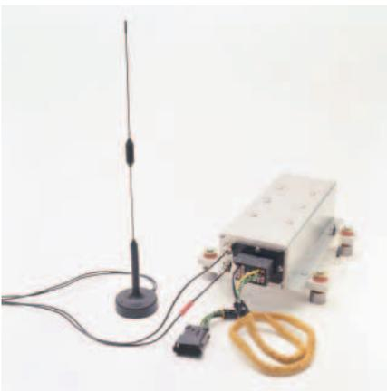
**Product Link.** The optional Product Link System is a factory installed or easily retrofitted wireless system that simplifies equipment fleet tracking. Using satellite technology, the Internet and your dealer's storefront website, the system automatically reports key machine parameters such as location, hour meter, active and logged service codes and forwards them to the customer through the dealer's storefront website.
