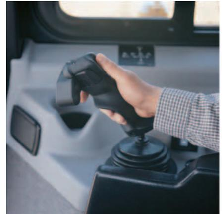
**Work Tool Controls.** The D6R II features ergonomically designed blade and ripper controls with low effort pilot operated hydraulics for added operator comfort, easy operation and precise work tool control. When equipped with a PAT blade, the blade control allows simultaneous six way control of the blade with a thumb rocker control to adjust blade angle.
