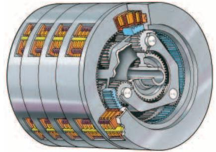
**Transmission.** The D6R II planetary power shift transmission features three speeds forward and three speeds reverse and utilizes large diameter, high-capacity, oil-cooled clutches. To maximize the life of the transmission, the planetary design distributes loads and stresses over multiple gears.
