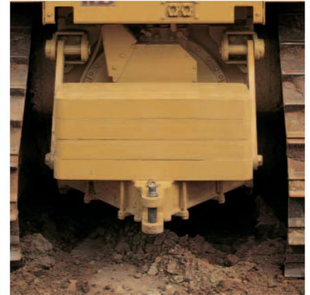
**Rear Counterweight.** Rear counterweights may be needed to optimize balance for backing up steep slopes or increasing performance in heavy dozing applications. Recommended if other rear attachment is not specified.
