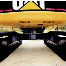
Carbody Design and Track Roller Frames. X-shaped, box-section carbody provides excellent resistance to torsional bending. Robot-welded track roller frames are press-formed, pentagonal units to deliver exceptional strength and service life.
