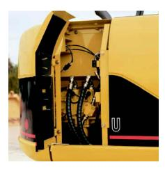
**Pump Compartment.** A service door on the right side of the upper structure allows ground-level access to the pump and pilot filter.
