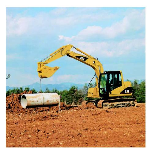
**Front Linkage.** Front linkage variations on the 311C U allow for the use of one boom, two sticks and five buckets. Using these combinations improves the general-purpose versatility of the 311C U by suiting it to a diverse range of applications.
