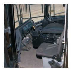
**Trainer seat.** The trainer seat consists of a padded seat and back with lap style seat belt. When the trainer seat is not in use, the back can be folded down and used as a drink tray and there is a storage compartment (room for a large lunch cooler) under the seat.
