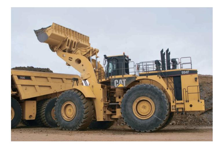
**Hydraulic System.** Completely enclosed hydraulic system uses separate circuits for lift and tilt, steering and brake control. Separate circuits provide increased cooling and elimination of cross-contamination, resulting in less downtime and greater productivity.
