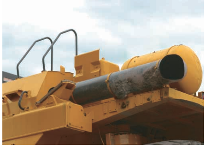
Muffler Housing and Walkway
