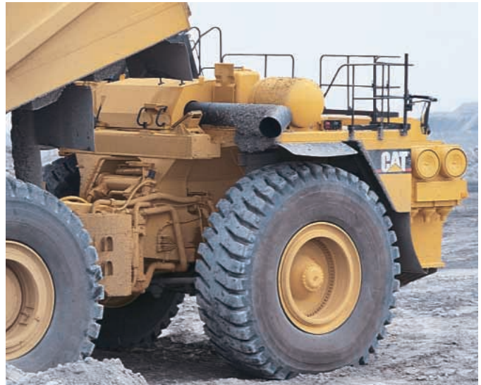
Muffler Housing and Walkway
