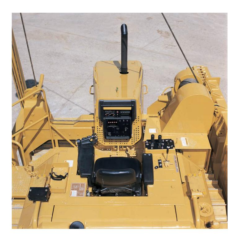
**Seat.** Ergonomically designed and fully adjustable for maximum comfort. The seat cushion reduces the pressure on the lower back and thighs while allowing unrestricted arm and leg movement.
