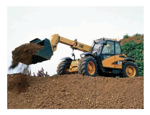
**Quick Coupler.** An IT interface is standard on the TH330B. For optimum versatility machines are equipped with a hydraulic quick coupler, allowing the operator to quickly and easily change non-hydraulic work tools without leaving the cab.
