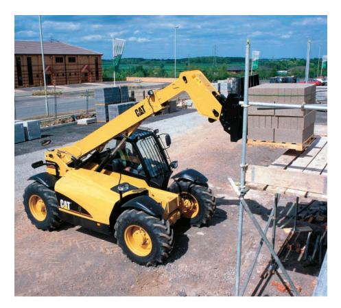
**Lift Height.** The TH330B can effectively and quickly place bricks and materials to a maximum height of 7.2 m (23.58 ft).
