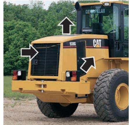
**Reverse Flow.** Air enters through the rear grill and exits out the top opening and side hood doors. Rear air flow picks up less debris from the ground, reducing plugging.
