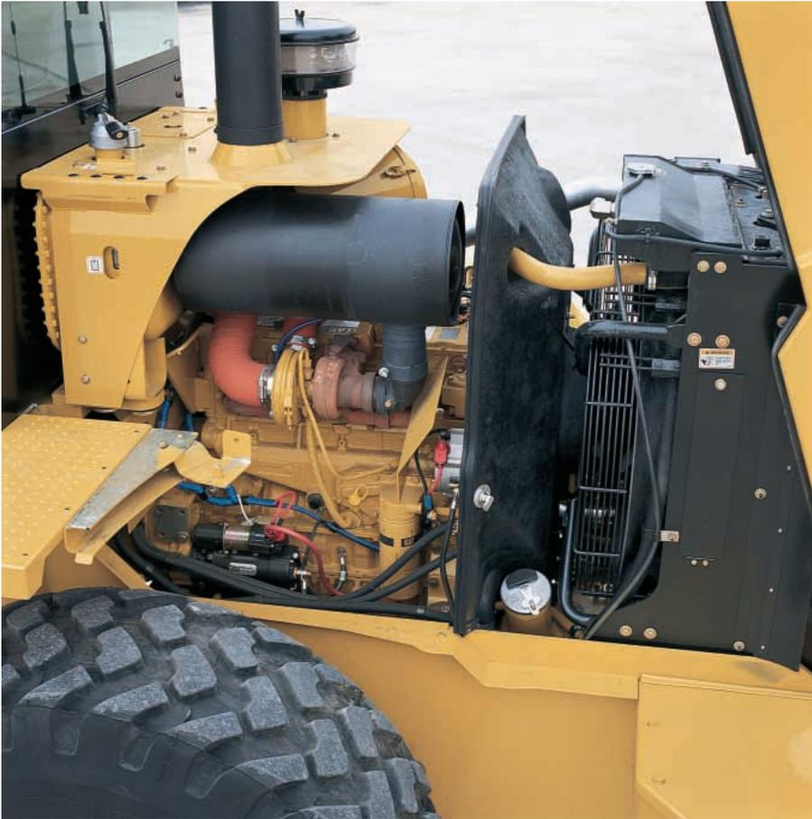
**Powerful Performance.** The 3126B ATAAC engine delivers net power of 119 kW (160 hp), and meets EPA Tier 2 emissions standards. Its advanced system keeps fuel at low pressure in the fuel lines until it is injected into the cylinder. Fuel pressure is created hydraulically in response to a signal from the ADEM III™ Electronic Control Module.
