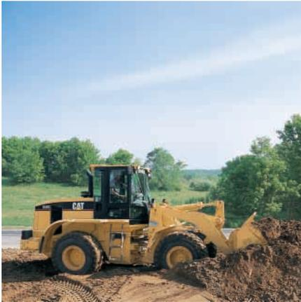
**Low Exhaust Emissions.** The Cat 3126B ATAAC engine used in the 938G Series II is a low emission engine designed to meet Tier 2 emission regulations. It is electronically controlled, with air-to-air aftercooling for more efficient combustion and cleaner emissions.
