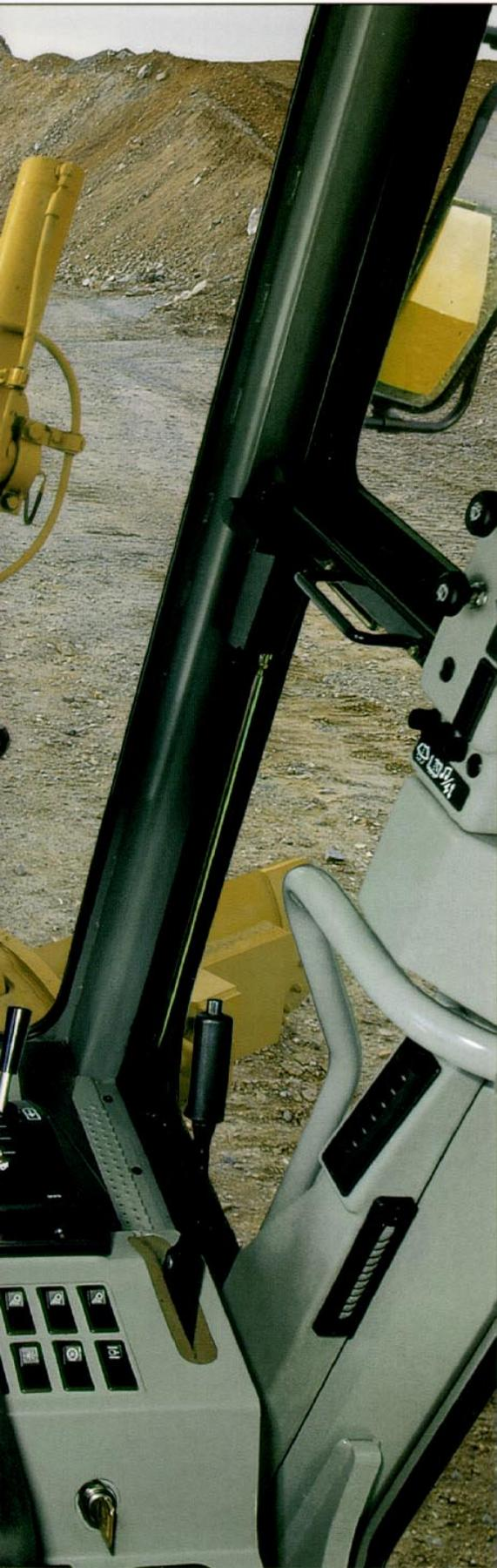
**Exceptional viewing area** helps improve operator confidence and productivity in all grader applications. The one-piece front windshield provides an unobstructed view of the work area. The large side windows offer a clear view of the moldboard heel and tandem tires. A wide rear window provides good visibility to the rear of the machine.
