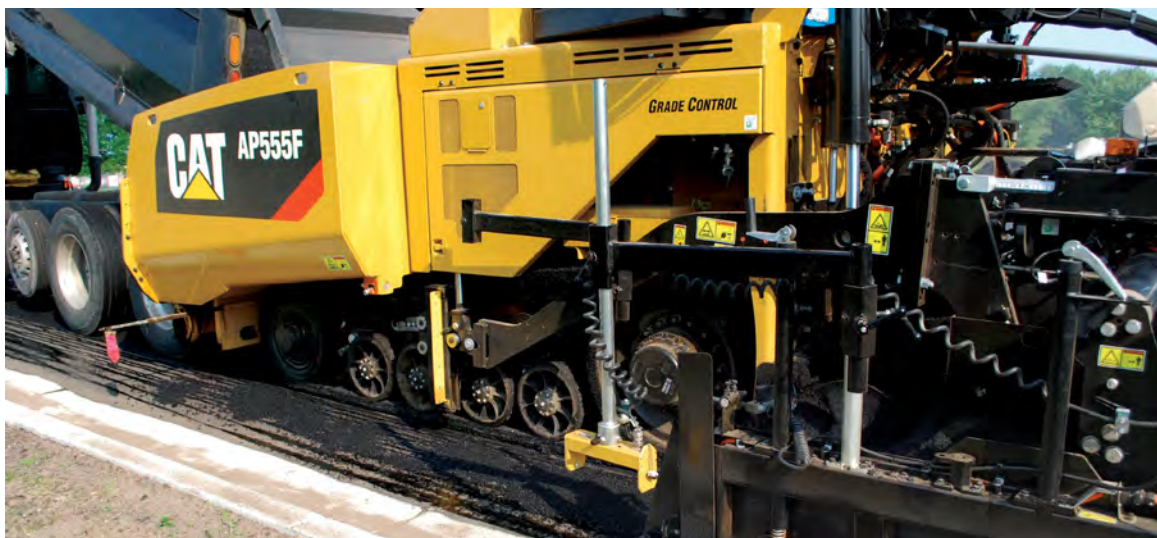
Set up grade and slope control according to project requirements or specifications.
