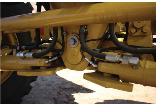
Front axle steering cylinder has been designed to enhance durability and hydraulic hoses have been routed to improve reliability.
