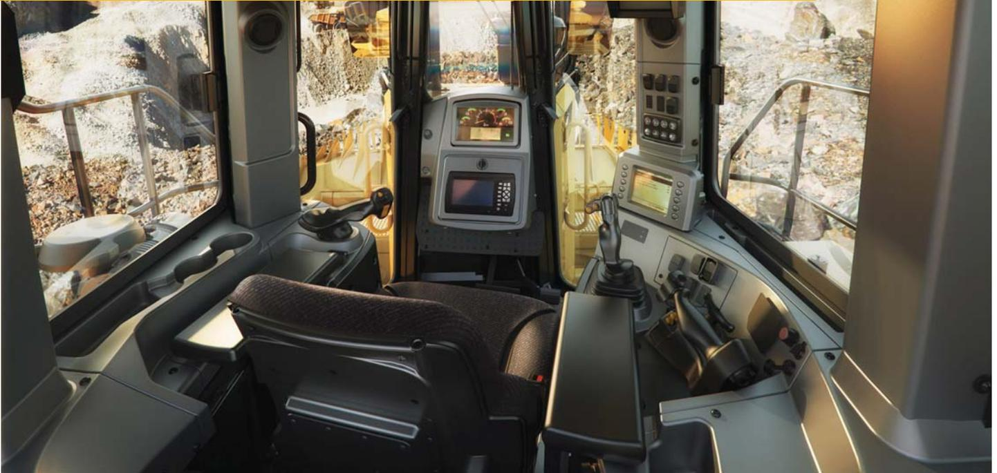
The D9T cab is designed and equipped for operator productivity, safety and comfort. The standard isolation-mounted cab reduces noise and vibration. Overall operator sound levels have been reduced by 2 dB(A).
