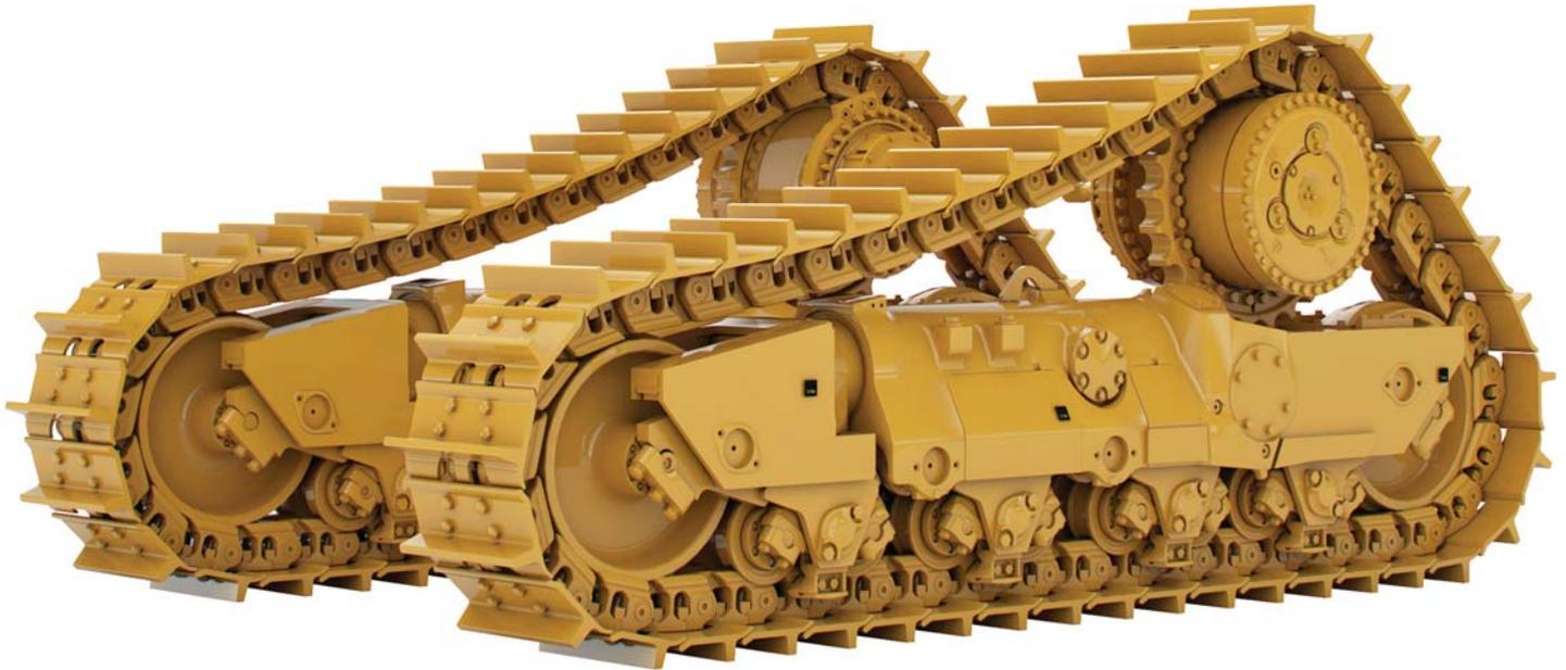
The elevated sprocket and fully suspended undercarriage work together, increasing traction while creating a smoother ride for your operators. The elevated sprocket design transfers impact loads to the mainframe, so final drives, axles and steering components are isolated from harsh impacts. These benefits translate into higher production and longer component life.
