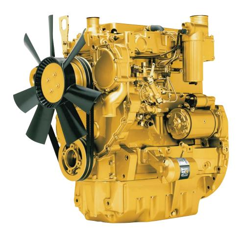
The Cat C4.4 engine has been designed to meet China Nonroad Stage III emission standards. This engine incorporates a time-proven mechanical governor and a low pressure fuel injection system which are major contributors to the improvement of fuel system robustness, high fuel efficiency and ease of troubleshooting. High filtration performance from the primary filter incorporating a water separator and a secondary filter also help to improve fuel filtration system reliability.
