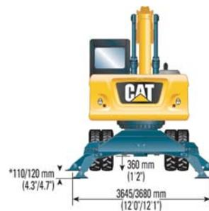
\*Maximum tire clearance with outrigger fully down
