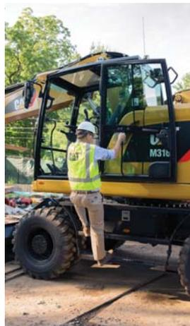
**Access into the cab** of a wheeled excavator has always been a challenge. We bring a solution to allow you to safely climb into the cab:
